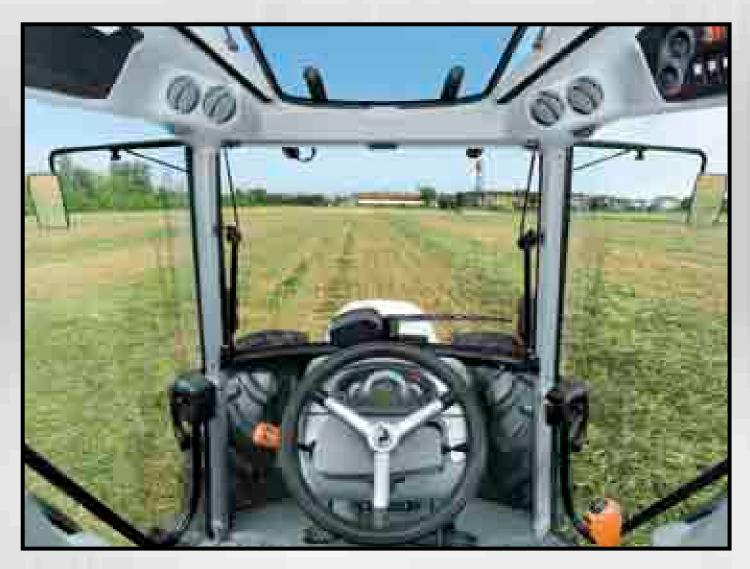
that a constant temperature will be maintained inside the cab, which is provided with a generous number of interior air vents adjustable for direction and flow.
