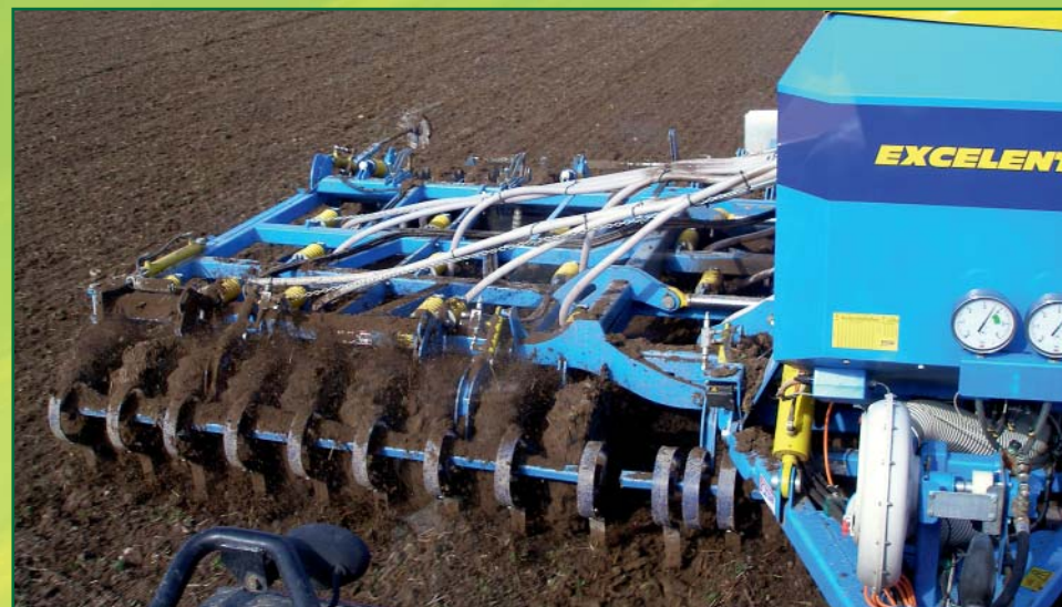
The short structure of the machine secures excellent copying and a small radius of rotation at the headland.
