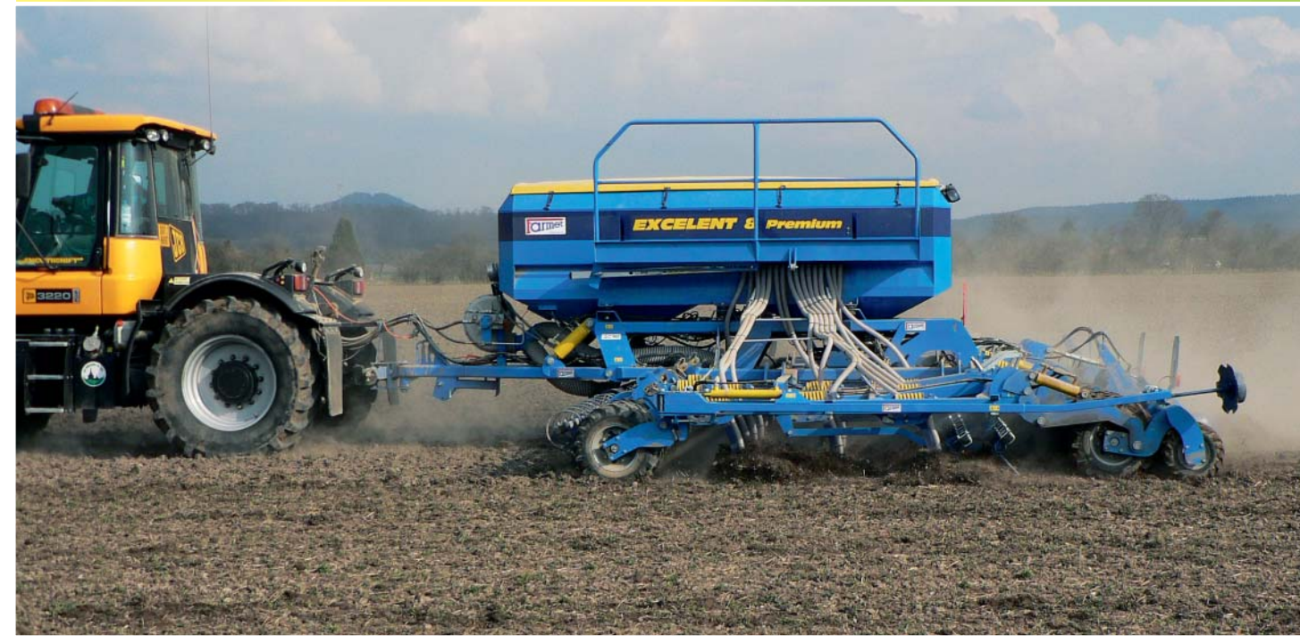
The short structure of the machine secures excellent copying and a small radius of rotation at the headland.
