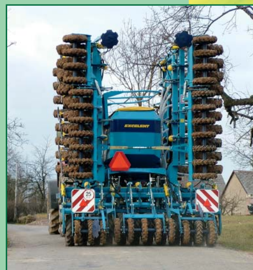
During transport, the small wheels of the rear tyre furrow presses are completely lifted. The travel wheels are protected against damage by PU foam.
