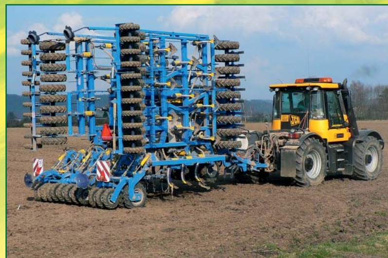
During transport, the small wheels of the rear tyre furrow presses are completely lifted. The travel wheels are protected against damage by PU foam.
