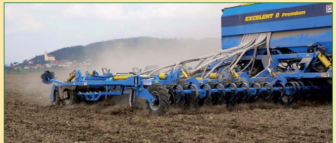
Front tyre roller in a combination with a hydraulically controlled finger skid excellently levels the soil and crushes the gobs.
