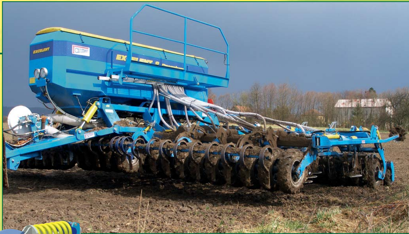
The semi-carried concept secures excellent manoeuvrability and trouble-free reversing.
