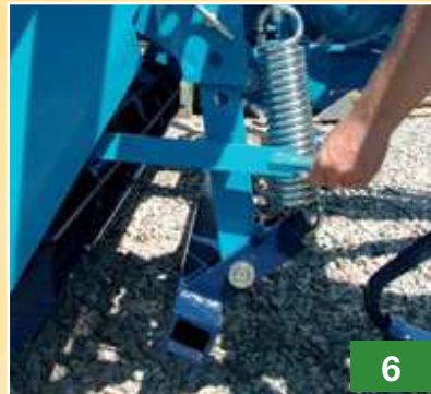
Front leveller board with a control lever for easy depth adjustment of the leveller.
