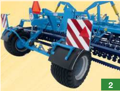
Wheels have tube [type] tyres. It is possible to fit the Kompaktomat with road lights for use on public roads.
