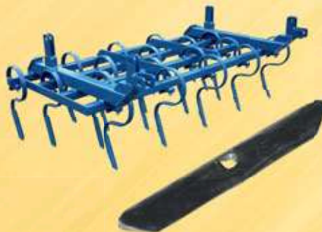
chisel point – width 45 mm
