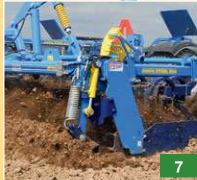
As a option, the machine may be equipped with hydraulically controlled front levelling boards.
