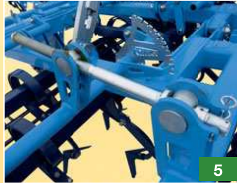
Mechanical depth control of working sections.
