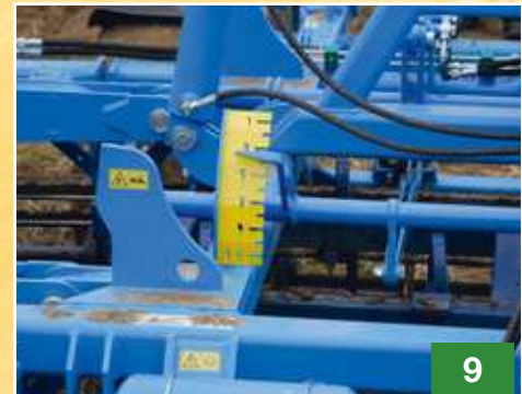
As an option, the working depth of the combinator can be controlled hydraulically from the tractor.
