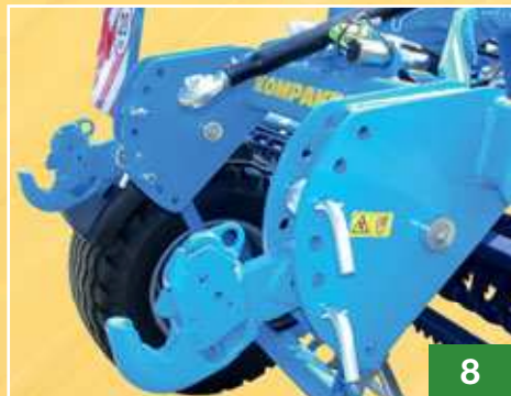
Semi-mounted machines may be equipped with a rear three-point hitch and piped for auxiliary hydraulic valves. Quick hitches [hook], category II, are provided.
