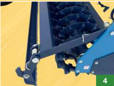
All crosskill rollers are made from very resilient cast iron withstanding work in very stony soils.
