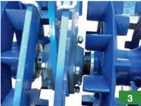
Rollers are fitted with longlife, greasable bearings.
