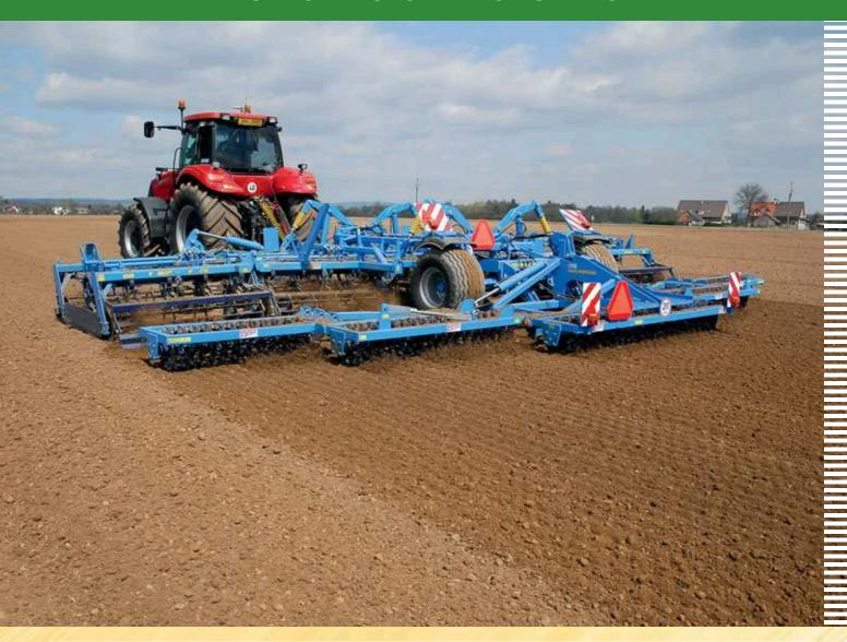
Optional crumbling crosskill rollers can be mounted on the rear three-point hitch of the Kompaktomat. These rollers can be used for further seedbed working if necessary, particularly in heavy soils. The rollers are lifted on the three-point linkage during transportation so they do not impair the manoeuvrability
